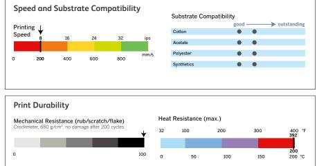
Videojet evaluation of observed performances of the Wash-resistant Ribbon with optimized printer setting and receptors.
